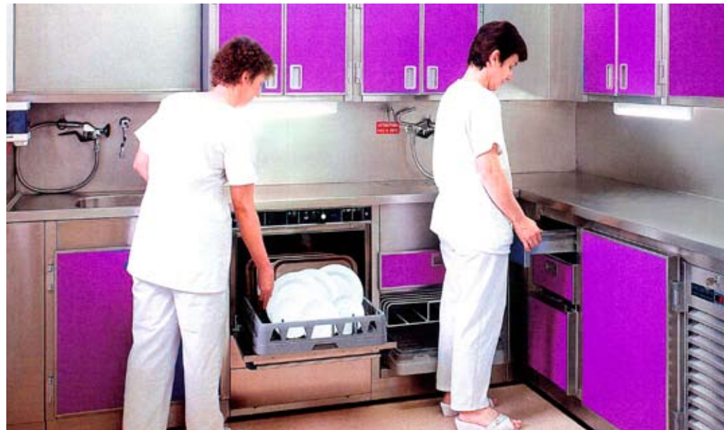
Drawers on telescopic slides are equipped with GN containers, which are dishwasher-proof
